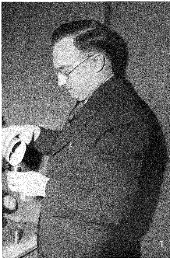
1. Tom pours green plastic powder into a mold around a part of the blade that failed. Heat and pressure applied by the machine directly behind him will mold plastic and the metal into a rod shaped piece about 1½" long 1" in diameter.
