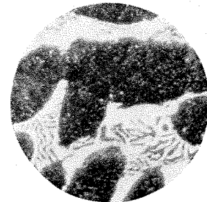
1000 times magnification of "AR" metal after heat treating with an air quench. The large dark areas are Martensite, the light areas Ceminite, with speckles of Austenite in the Martensite. These are three of the numerous metallic structures.
